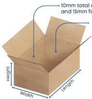
10mm total clearance on side for one row and 15mm for multi-row packing.
