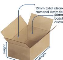
10mm total clearance on side for one row and 15mm for multi-row packing.
