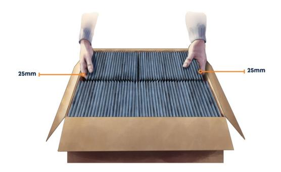
With the ERGOSA in horizontal mode your packing personel will pack a long batch of boxes in one fast sliding movement. The case must have 25mm clearance on each end, when the batch is compressed, to accommodate the hands without scraping the knuckles.
